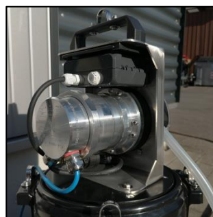
Sampling module in the non Ex version with small Li-Ion rechargeable battery
