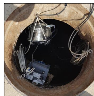
EX-version of the sampling module, installed in the manhole
